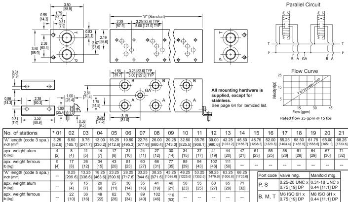
\* Length of 01 station with relief cavity is 4.50 [114.3]. Gauge port not available on 01 station.
